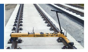
SLAB TRACK CONSTRUCTION CALLS FOR FAST, PRECISE MEASUREMENTS, AND IMMEDIATE FEEDBACK. THE TRIMBLE GEDO SYSTEM LETS YOU MEASURE FOR PRECISE ADJUSTMENTS, INSPECTIONS, AND QUALITY CHECKS. IN ONE OPERATION, THE TRIMBLE GEDO SYSTEM CAPTURES 3D COORDINATES OF THE TRACK, TOGETHER WITH GAUGE AND CANT. THE INFORMATION IS COMPARED TO THE DESIGN, AND OFFSETS AND CORRECTION VALUES ARE DISPLAYED IN THE FIELD, WHERE WORK CREWS MAKE THE NECESSARY ADJUSTMENTS.
