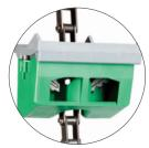
The grain property bucket is the key to our single calibration. By throwing extra grain across the sensor one time per chain rotation, it enables YieldSense to accurately report yield as kernel properties and moisture levels change.
