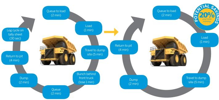
Typical haul truck cycles include many inefficient tasks and delays
